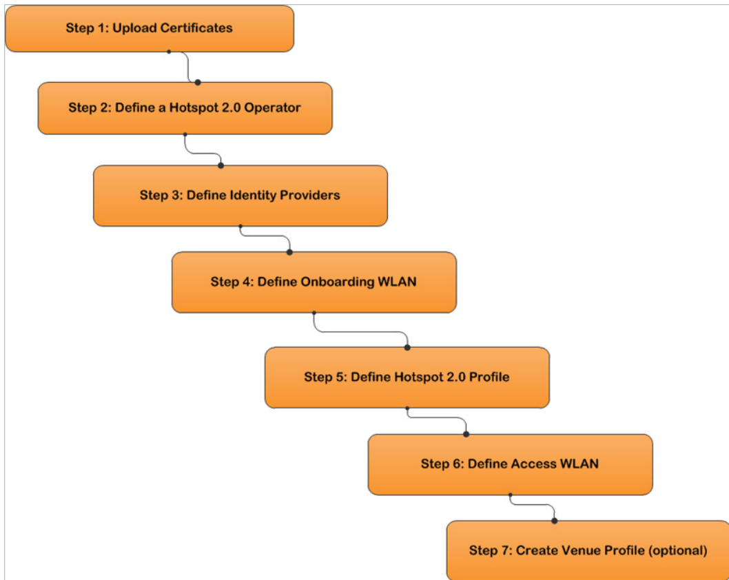
Figure 3. Hotspot 2.0 Configuration Flow
